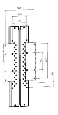
Plasma/LCD mounting bracket for use with TS460. Powder coated in RAL 9006 (alu-look). Weight capacity 50 kilos.
